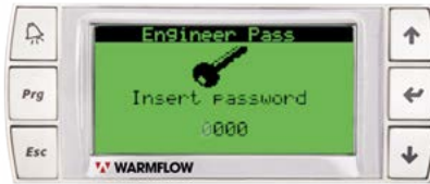
Figure 19: Engineer Pass Screen.
