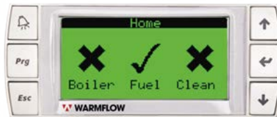
Figure 77: Home Screen – Alarm Condition
