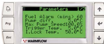
Figure 68: Engineer Parameters Screen 1
