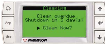
Figure 26: Cleaning Status – Overdue
