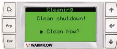
Figure 27: Cleaning Status – Shutdown
