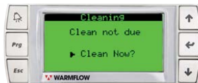
Figure 24: Cleaning Status – Not Due
