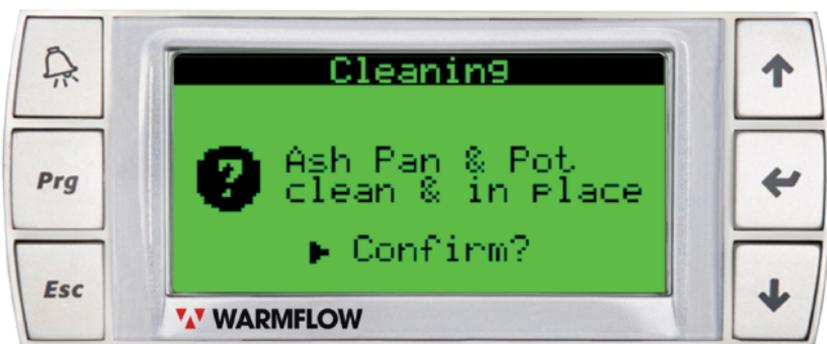
Press the enter key to confirm that the ash pan and combustion pot have been cleaned and put in place. The boiler will return to the home screen with the clean icon now showing as a tick. Should the controller indicate that the combustion door is open, the door handle has not been pushed down fully. Please return to the boiler and ensure that the handle is pushed down firmly.
