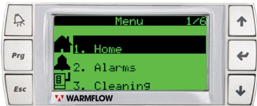
**Main Menu** - The main menu (accessed via the menu key) can be scrolled using the up and down keys and will allow you to navigate the menu.
